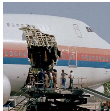
Rapid Decompression Load
