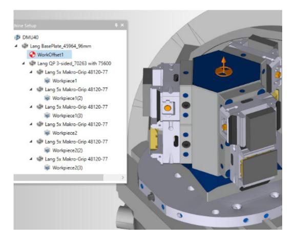
The work offset definition enhancement in ESPRIT 5.1 lets you define a work offset directly on the machine or on a fixture, share a work offset between multiple workpieces, and program a unique main offste with dynamic offsets.
