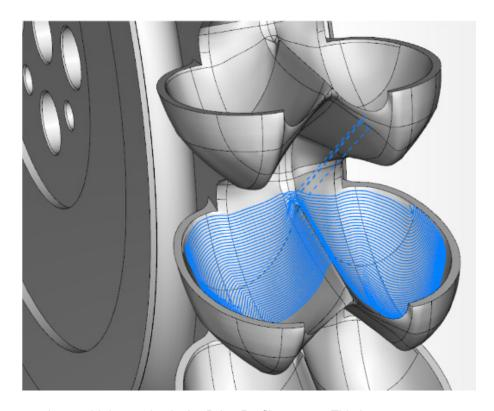
Now offered for composite machining cycles is the Drive Profile pattern. This lets you generate passes from selected geometry, without the need to create a drive surface.
