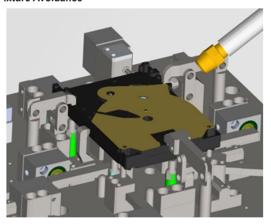
This new option for pocketing cycles lets ESPRIT automatically detect and eliminate toolpath segments that will cause collisions with the tool or fixture assemblies, with no need to create extra geometry to constrain the toolpath or alter fixture data in the ESPRIT document.
