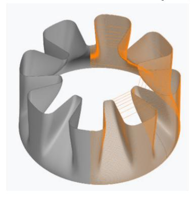
This new additive cycle lets you create walls from surfaces sliced along the Z Axis. Create these cycles from open or closed faces and from any substrate shape. Build several faces simulaneously with sub-feature compatibility.
