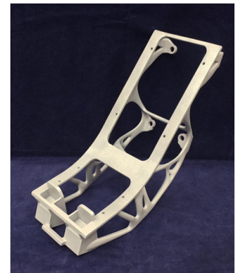
The optimized casting.
