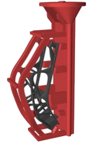
The gating design created by Solidiform.
