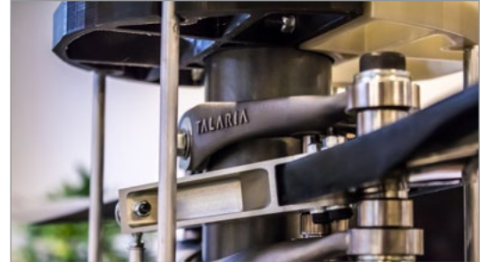
The topology optimization of the rotor hubs resulted in a weight reduction of almost 30%.
