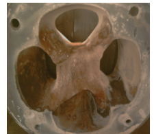
Tool Damage from Excessive Cycling
