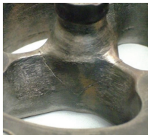
Tool Damage from Deflection
