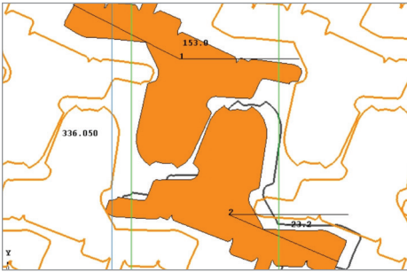
Blank nesting to maximize material utilization
